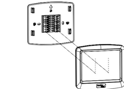
Figure 3. Mount thermostat to wallplate
