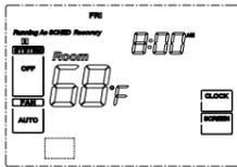
1) The display indicates "STD2" (default for multi-stage mode) in the display. Select the system "SS1", "HP1" or "HP2" by pressing the up or down key. In "SS1" and "STD2" configuration, EMER mode is useless.
