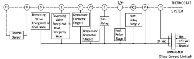
Figure 7. Typical wiring diagram for single transformer multi-stage systems
