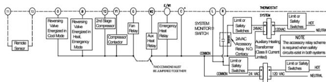
Figure 6. Typical wiring diagram for two transformer heat pump systems with safety circuits in BOTH systems
