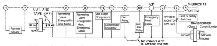
Figure 5. Typical wiring diagram for two transformer heat pump systems with NO safety circuits
