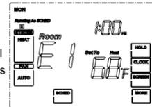
battery with two new AAA alkaline battery, even if you have recently replaced them. Move the battery out, and then hold any key to release the rest energy. Then place the battery again. You will need to reprogram your thermostat and confirm normal operation. If Error Mode returns, please call us for further information.
